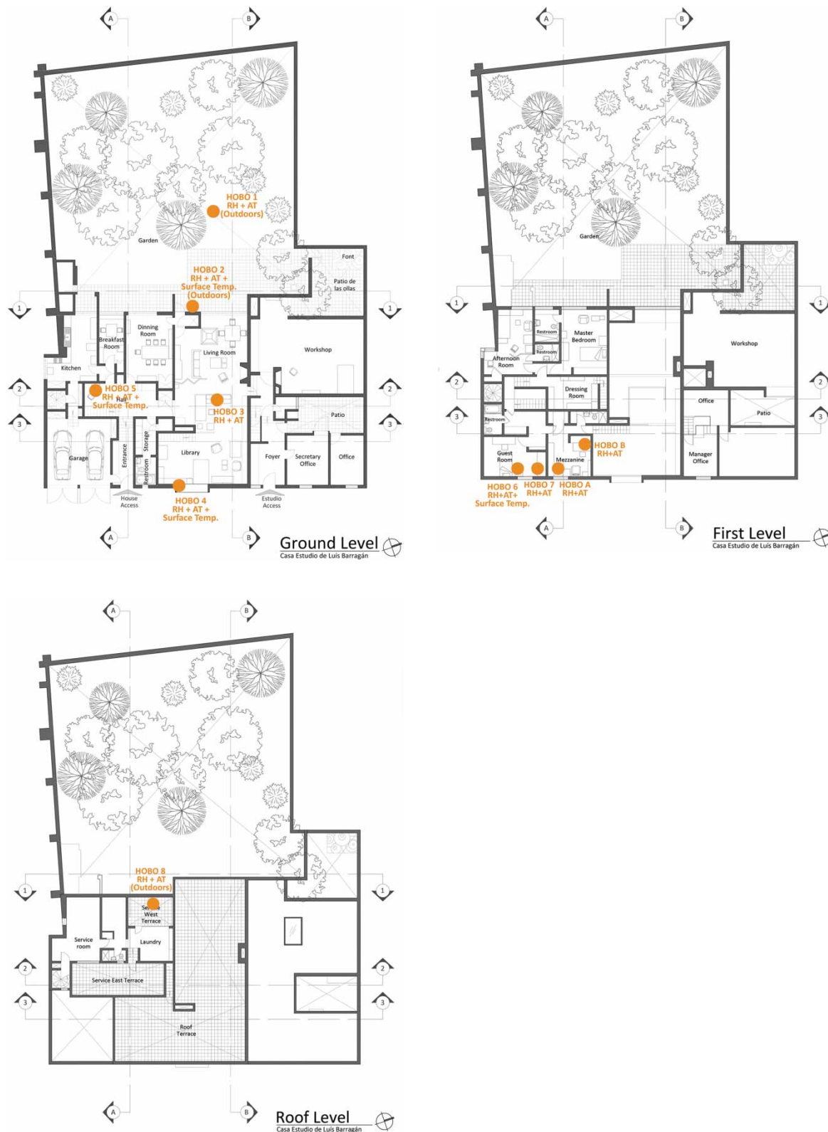
Figure 2. Floor plans of La Casa de Luis Barragán (Redrawn after http://www.casaluisbarragan.org/planos.html ). Location of temperature and humidity sensors are shown in the plans. © [Catalina Corcuera]. Reproduced by permission of Catalina Corcuera, Director, Casa Luis Barragán.
